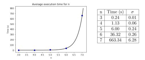
Figure 2: Runtime of the one controlling-qubit period-finding algorithm over different values of n. The specific N values used were 7, 15, 25, and 35, respectively.
