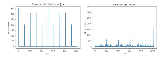
Figure 1: Distributions of  $|c\rangle$  from Shor's quantum period-finding algorithm, with N = 25, Q = 1024, y = 4, and r = 10. The left graph shows the expected distribution of  $-c_{\dot{c}}$  outputs, while the right graph shows the actual distribution when following the implementation given in [1].
