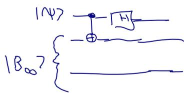
$|\Psi_2\rangle = \frac{1}{2} [ |00\rangle(\alpha|0\rangle + \beta|1\rangle) + |01\rangle(\alpha|1\rangle + \beta|0\rangle) + |10\rangle(\alpha|0\rangle - \beta|1\rangle) + |11\rangle(\alpha|1\rangle - \beta|0\rangle) ]$
