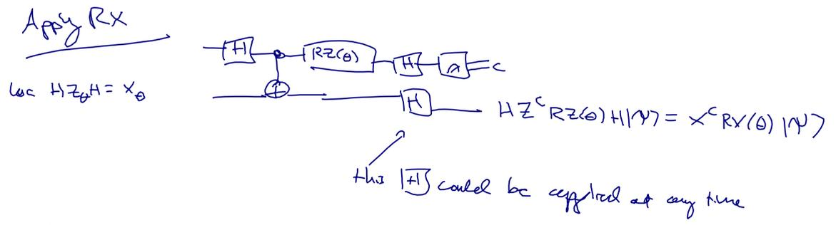
Thus we are universal for single qubit gates because any  $U = R_x(\alpha) R_z(\beta) R_x(\gamma)$  for some  $\alpha, \beta, \gamma$
