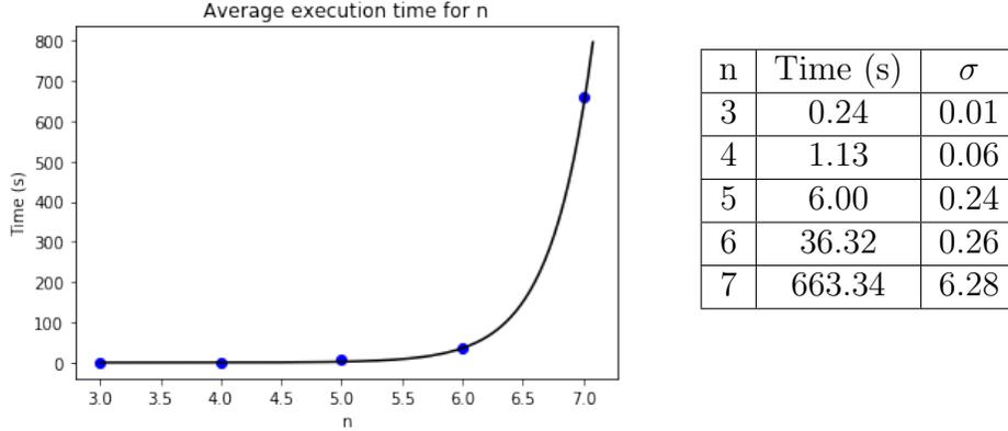
Figure 2: Runtime of the one controlling-qubit period-finding algorithm over different values of  $n$ . The specific  $N$  values used were 7, 15, 25, and 35, respectively.
