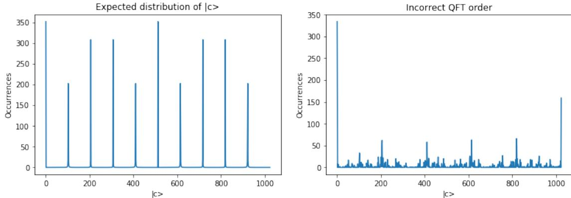
Figure 1: Distributions of  $|c\rangle$  from Shor’s quantum period-finding algorithm, with  $N = 25$ ,  $Q = 1024$ ,  $y = 4$ , and  $r = 10$ . The left graph shows the expected distribution of  $|c_i\rangle$  outputs, while the right graph shows the actual distribution when following the implementation given in [1].
